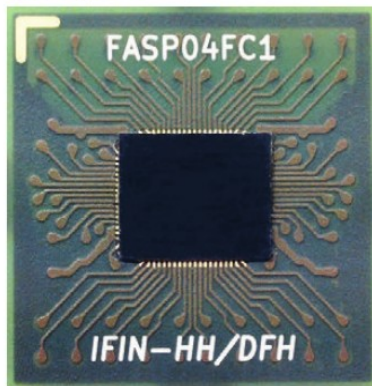
Fig.2: FASP_04 PCB substrate for flip-chip connection.
